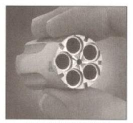
Hammer safety slots in between cartridge chambers
